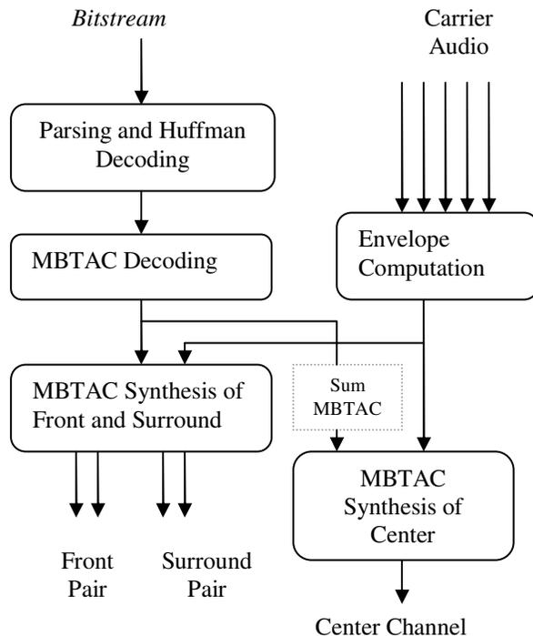
Figure 4: 8 – 12 Kbps Mode Decoder (Partial)
