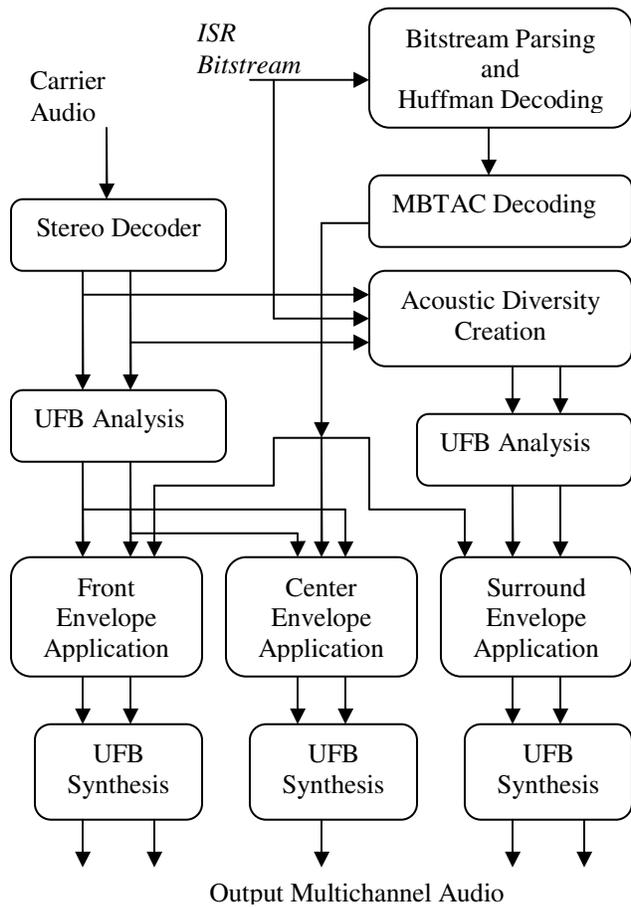
Figure 3: ISR Decoder Architecture
