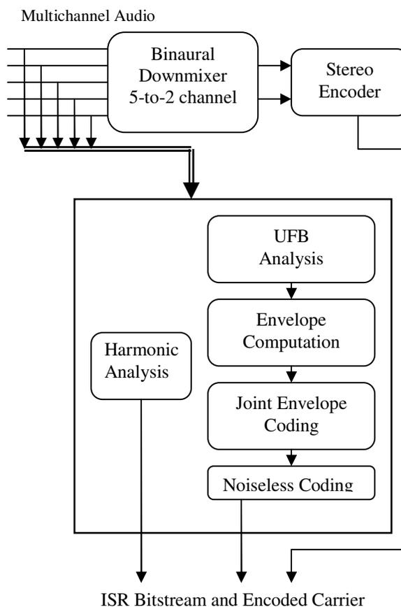
Figure 1: ISR Encoder Architecture
