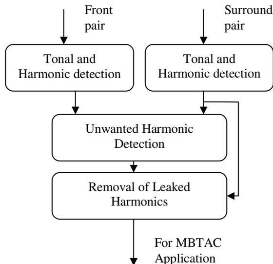
Figure 2: Acoustic Diversity Creation through Harmonic Removal
